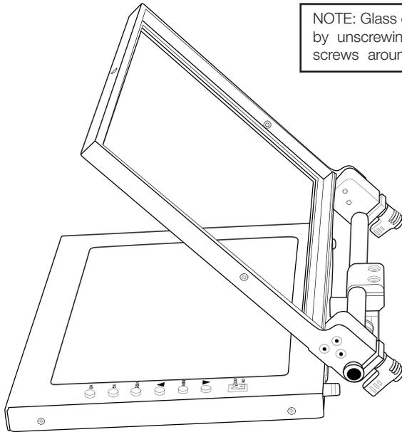
NOTE: Glass can be removed by unscrewing the three (3) screws around glass frame.
